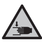
Warning crushing of hands
